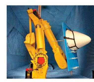
Applied Composites also offers transmissivity testing on a "test-only" basis for customers with internal repair capabilities
